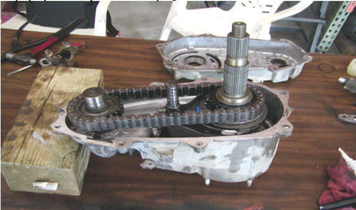
Photo 4. NP231 after completion of the first 9 steps. The rear case half is now ready to be installed.
