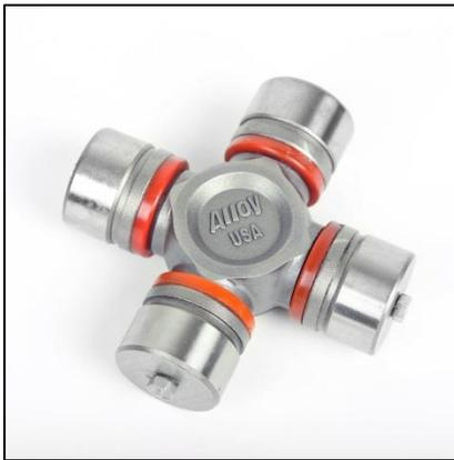
Available for Wrangler Rubicon and Rubicon Unlimited models equipped with Super Dana 44 axles, the heavy-duty X-Joints are a direct replacement for the factory U-joints. The X-Joints are manufactured from 8620 case hardened alloy steel and incorporate a number of design features to ensure the joints stand up to the stresses of off-roading.
