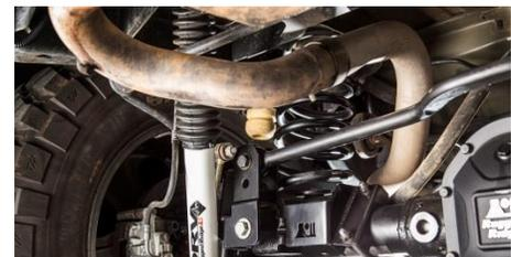
Rugged Ridge Rear Track Bar Relocation Bracket restores proper track bar positioning on lifted JK Wranglers.
