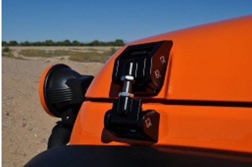
Above: The black powder coated billet aluminum JK Wrangler hood Catch kit from Rugged Ridge
