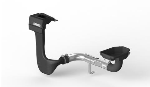
The standard Modular XHD Snorkel System comes with a low-mount intake that is located away from the front of the vehicle, a safer position that prevents dangerous exposure to water during fording of rivers and streams. An optional high-mount 'ram' accessory moves the air intake up an additional 21-inches to the top of the windshield for deeper water crossing. The new design also benefits from the ability to draw cool air from outside the hot engine bay where the factory air box is located.
