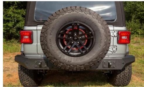
The LED Third Brake Light Ring provides improved positioning for greater visibility, especially on lifted Jeeps.
