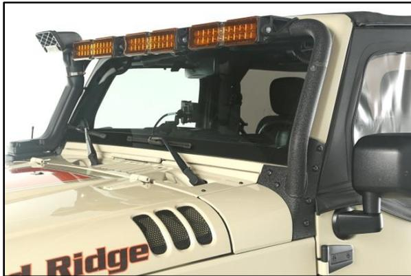
Rugged Ridge’s new LED Light Bar Mount features a unique contour hugging design that requires no drilling whatsoever for easy installation. **Photo Credit:** Omix-ADA
