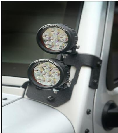
Rugged Ridge's new A-pillar mounted LED light brackets accommodate two additional round or cube-style lights and are engineered for easy installation, requiring zero cutting or drilling.
