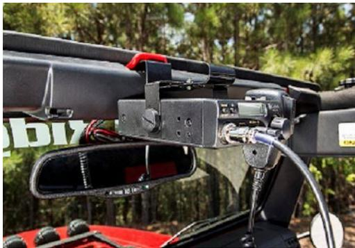
Rugged Ridge's new CB Radio Mount for 03-06 Wrangler TJ/LJ attached the unit to the upper windshield frame for increase security.
