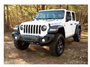
Rugged Ridge's unique stamping process makes the Spartacus Stamped Steel Front Bumper one of the lightest aftermarket bumpers around.
