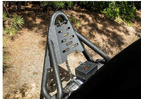
Since the Rugged Ridge XHD Stinger Guard is designed specifically for the Rugged Ridge XHD Stinger, installation is simple with only minimal drilling required and all mounting hardware and instructions included. The XHD Stinger Guard will allow for full use of the XHD Stinger Winch Hook Holder when properly installed, preserving all of its functionality, but with a new and integrated look.
